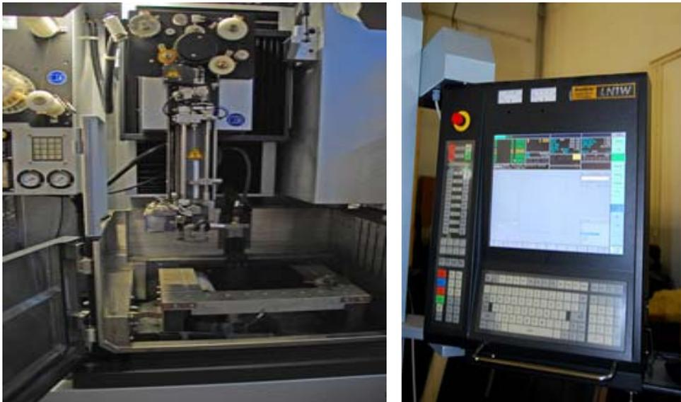
**Figure 2** Electrical erosion machine Sodick wire AQ300, equipped on LN1W CNC.
