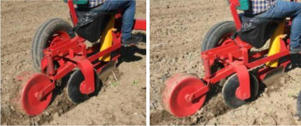
**Fig. 2** The working process carried out by the miscanthus rhizomes planter section
