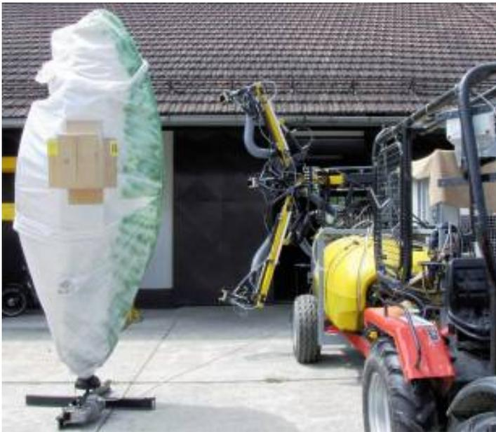
**Figure 4** Laboratory testing based on LIDAR measurements of a solid model of a tree
