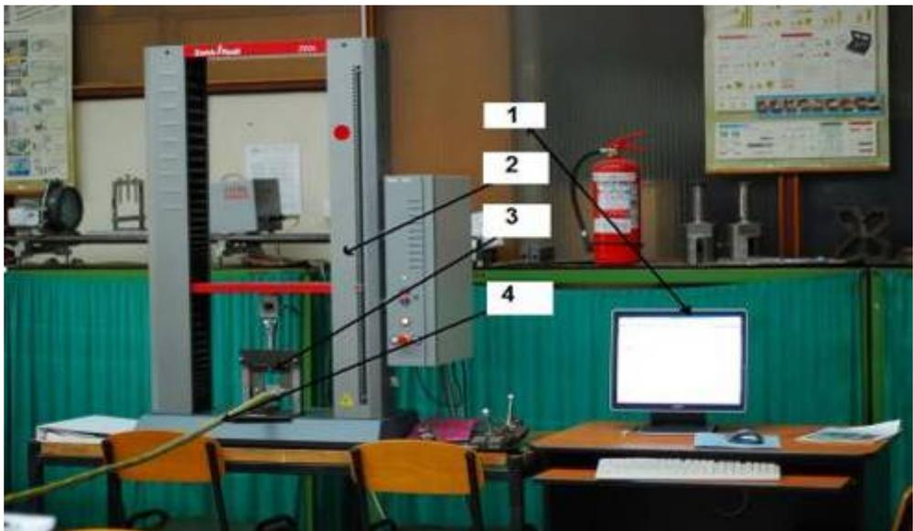
**Figure 2** Working stand used for determination; 1 – Unit for recording and processing of the experimental data, 2 – Zwick/Roell Z005 Static material Testing Machine, 3 – SRC’s cutting tool, 4 – Sample (energetic willow stem); The method’s testing integrated equipment requires a special cutting tool for SRC.
