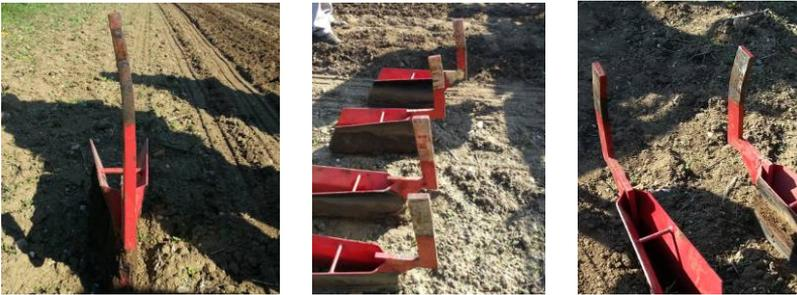
**Fig. 13** Working organs supports irreversibly deformed during the forced working regime
