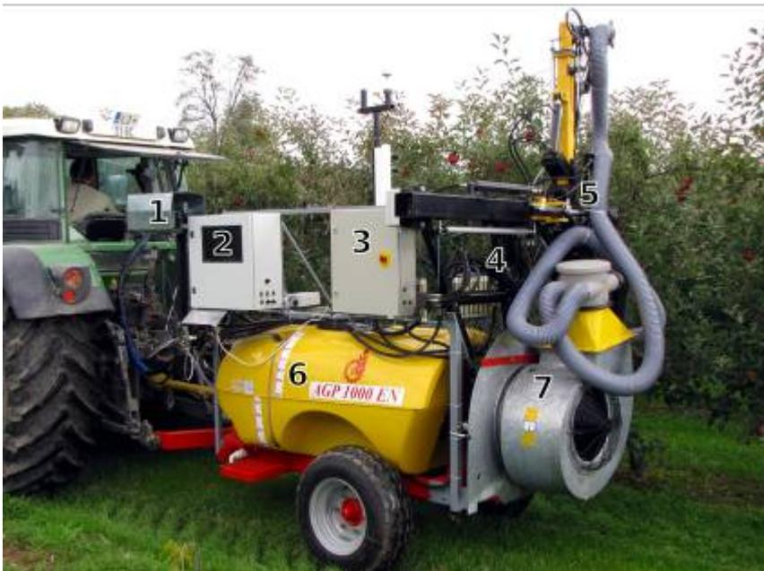
**Figure 2** Sprayer with sensors and manipulators (1 - LIDAR with protective housing, 2 - computer box, 3 - electronics box, 4 - electromagnetic valves, 5 - sprayer arms and air ducts, 6 - basic sprayer, 7 - radial fan)
