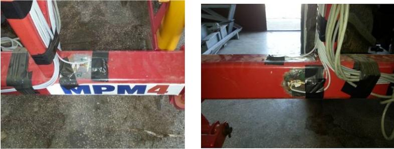
**Fig. 12** Locations of strain gauges - details
