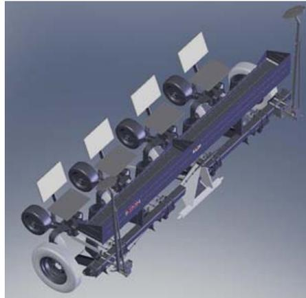
**Fig. 1** Spatial drawing (3D) of the assembly of the Miscanthus planting machine, MPM-4
