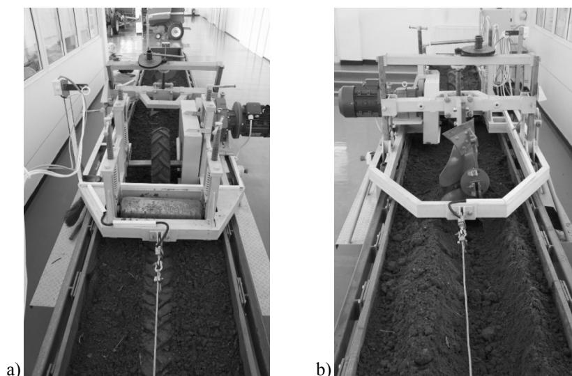
Fig. 2 Laboratory experiments in order to study of the interaction of tire wheel and active part with the soil: a – study of the wheel -soil interaction; b – study of the plough body - soil interaction
