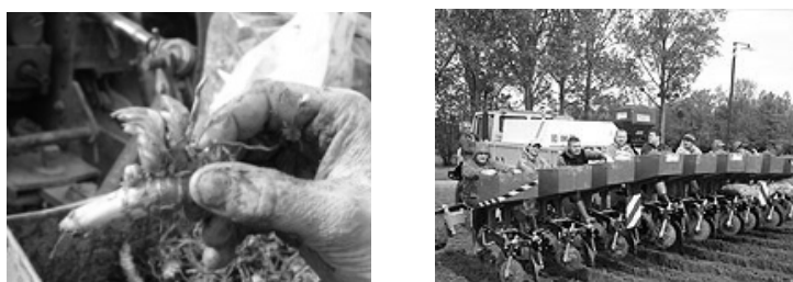
Fig. 6 The Miscanthus planting machine adapted from the potato planting machines [13]
