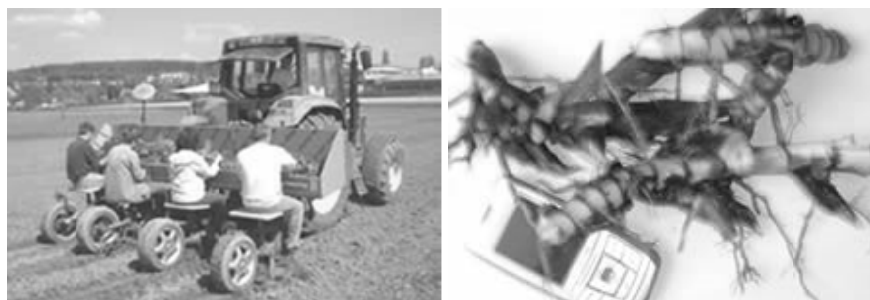
Fig. 4 Semi-automated miscanthus planting machine [12]
