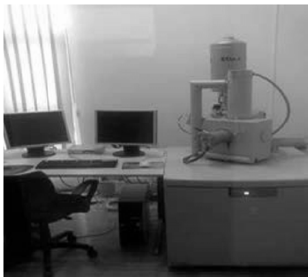
Figure 1 Scanning electronic microscope Inspect S. (National Institute for Electrochemical and Condensed Materials of Timișoara)
