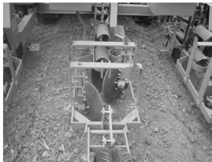
Fig. 8 NORDIC rhizome planting machine design [5]
