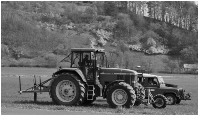
Figure 2 Horizontal penetrometer during measuring on the field
