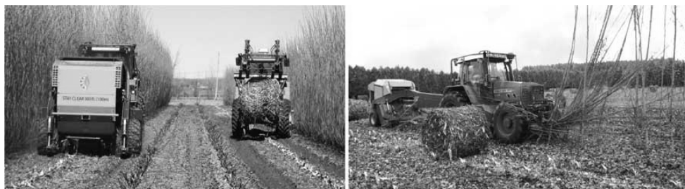
Sl. 1 Stroj BioBaler WB 55 proizvođača Anderson Group co. u berbi-sječi vrbe Fig. 1 Anderson Group co. BioBaler WB 55 harvest biomass in short rotation crop of willow
