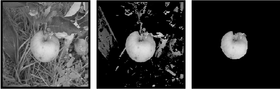
Figure 1 A test example – the left image presents the original images of a natural scene, the middle image its colour segmented version and finally, the right image, the result that was confirmed 2D or 3D shape analysis
