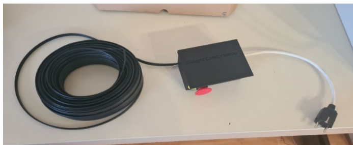
Figure 8. Heating cable system with controller
