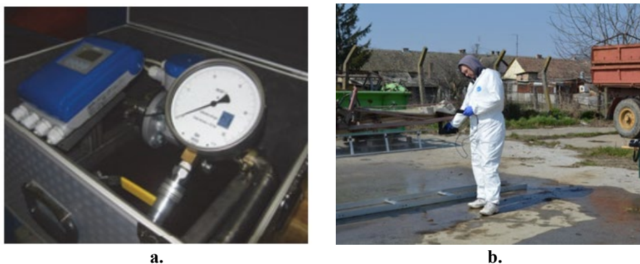
Figure 1. Ultrasonic pump capacity tester (a.) and nozzle flow testing (b.)
