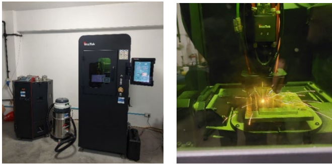
Figure 7. Metal-based additive manufacturing with DED
