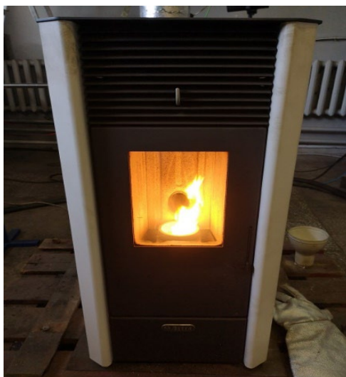
Figure 6. Pellets combustion test: Pellets burned well and burning efficiency was high
