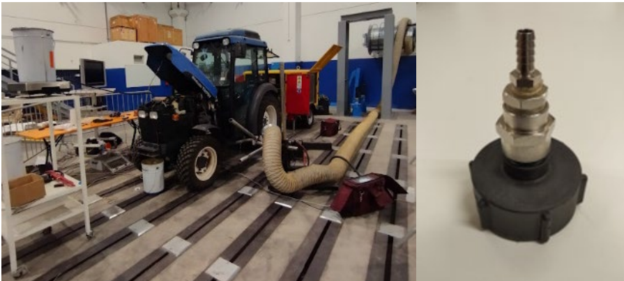
Figure 1. Engine Tractor test bench and modified tractor tank cap
