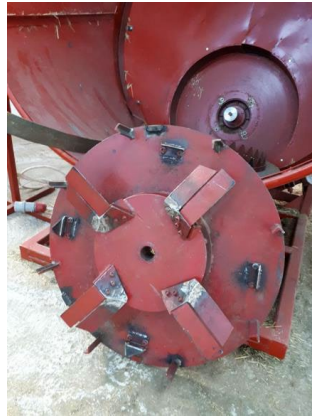
Figure 1. Miller and shredder assembly V1 (Cenei Industrial Park)
