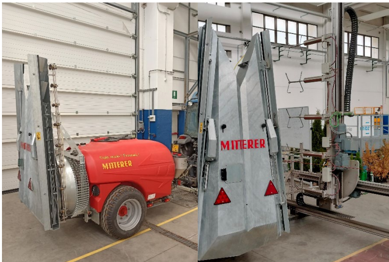
Figure 1. The employed sprayer (left). Notice the top deflector at the upper end of the distribution system. On the right is a detail of its air distribution system with the WP5000 sensing array.
