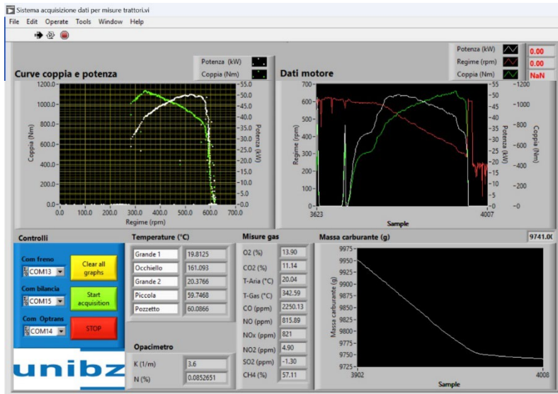
Figure 2. NI LabView interface for the tractor engine acquisition data
