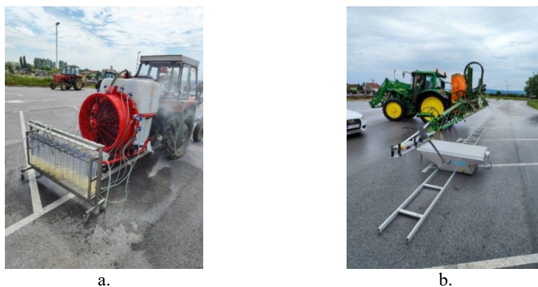
Figure 3. Nozzle flow and liquid distribution check
