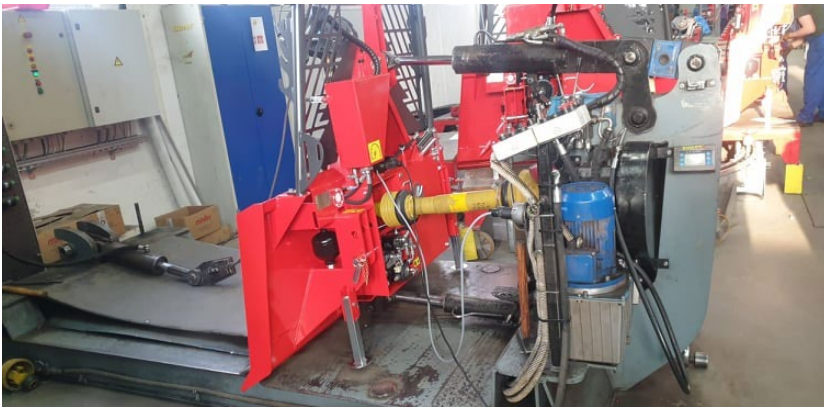
Figure 1. Device for testing the pulling force of a winch
