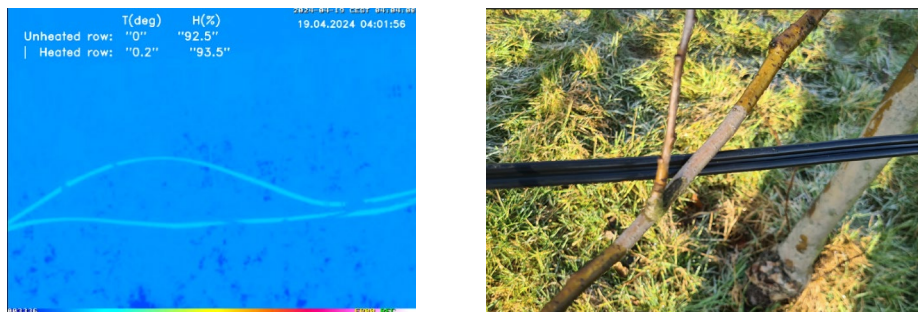
Figure 14. Thermal image of the heating wire captured by MOBOTIX combined with an RGB image
