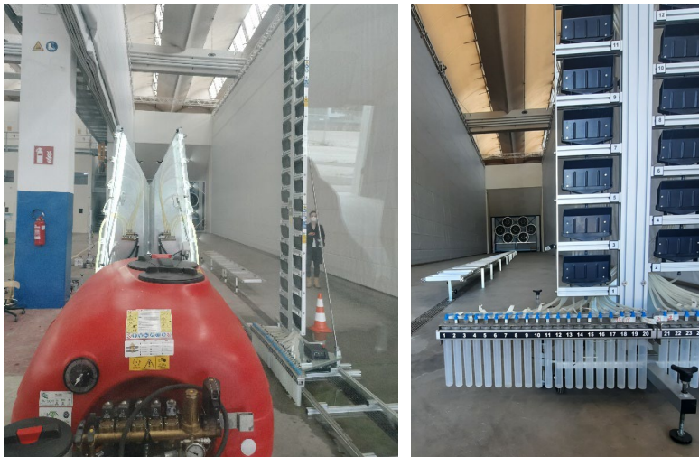
Figure 2. The sprayer during a deposition test on the vertical patterator (left) and a detailed view of the patterator (right). The collecting surfaces in black convey the liquid to the graduated tubes at the bottom.
