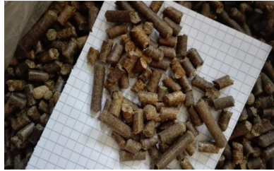
Figure 6. Sample of straw pellets obtained with the pellet line
