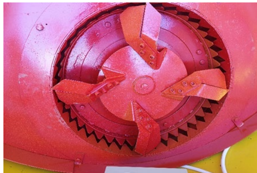
Figure 2. Miller and shredder assembly V1 (Cenei Industrial Park)
