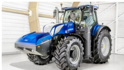
Figure 1. A tractor that can run on CNG or biomethane, an additional gas tank is also mounted on the front of the tractor (source: New Holland).
