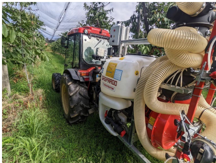
Figure 1 The airblast sprayer Turbo Teuton P Polipo with a built-in spraying sensor system
