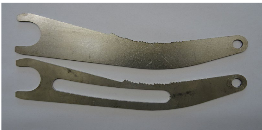
Figure 1 Original seed eliminator (down) and new seed eliminator (up)
