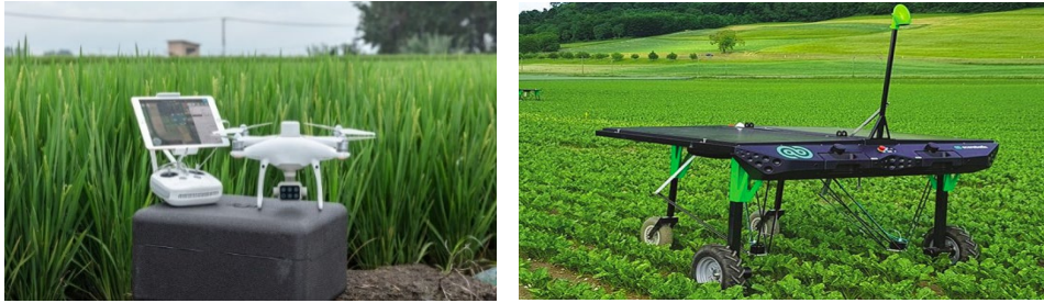
Figure 7 P4 Multispectral (DJI) UAV (DJI, 2019) and Ara robot from EcoRobotix (right)
