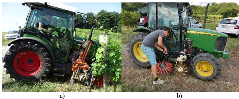
Figure 1 Braun tools for control of weeds underneath vines in the vineyard a) LUV Perfect grass trimmer - ploughshare undercutter mounted on side of tractor (locally called Lama) and trunk cleaner attached on side of mulcher, b) rotating star hoe (in german called Rollhacke) and trunk cleaner monuted on side of mulcher.
