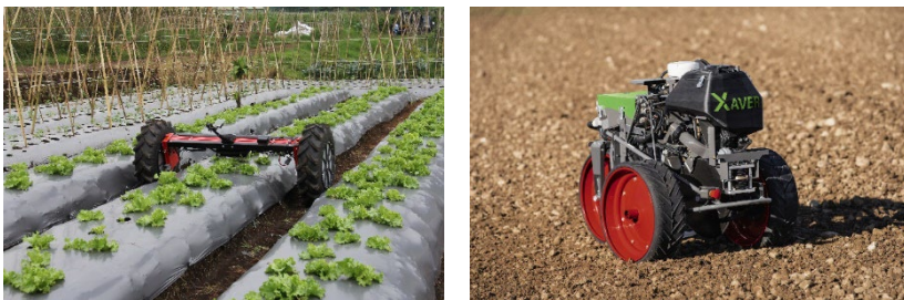
Figure 4 Di-Wheel robot (Sukkarieh, 2017) and Xaver Sowing Robot (Fendt, 2020)
