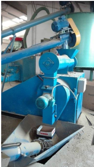
Figure 1 Technological line for the production of pellets
