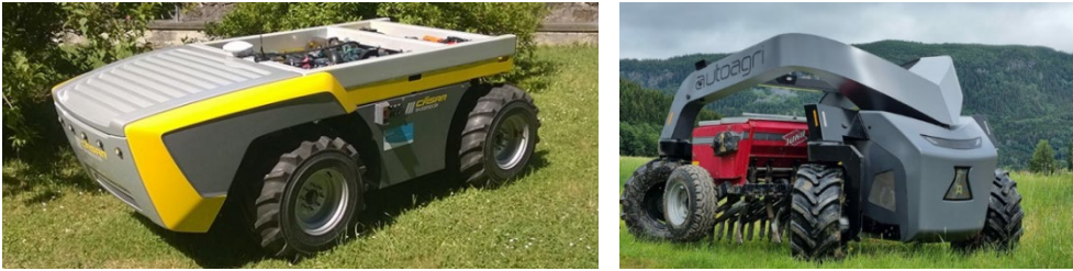
Figure 3 Cäsar robot (Raussendorf GmbH, 2017) and ICS 20 robot (AutoAgri, 2021)
