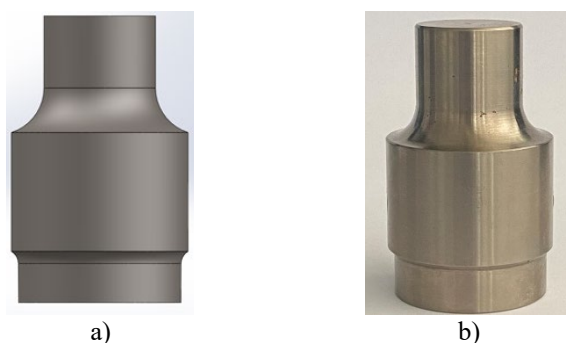
Figure 6 The construction details of the sonotrode designed for the extraction of volatile oils from sea buckthorn: a) 3D model sonotrode; b) fabricated sonotrode
