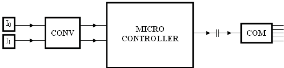
Fig. 4 Principle scheme of the data acquisition system using a microcontroller
