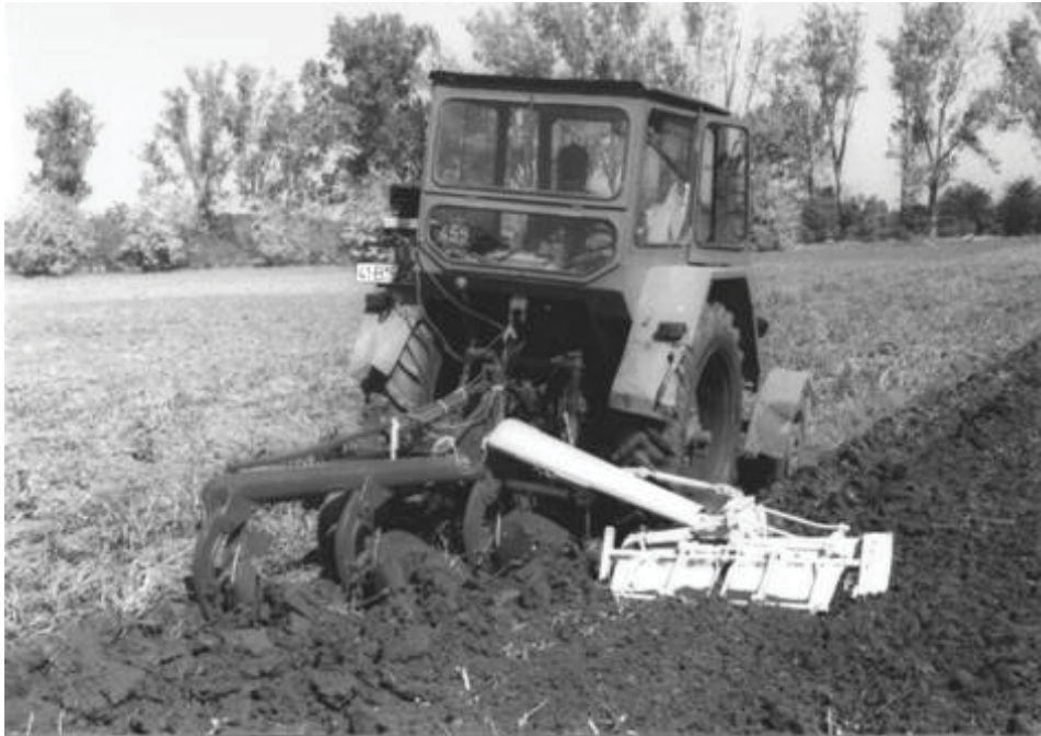
Fig. 5 The tillage cutter works at an angle towards the tractor's longitudinal axle
