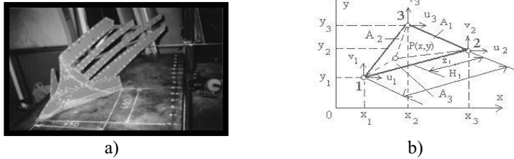
Figure 1 a) The studied Lemken lamellar moldboard. - b) - The studied triangular finite element
