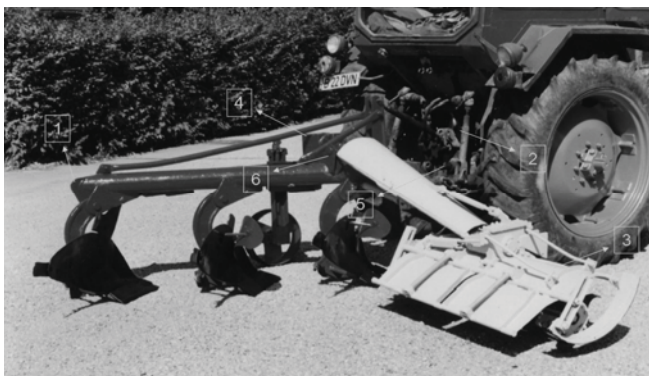
Fig. 1 Soil preparation experimental unit: 1 – suspended plough; 2 – three-point linkage; 3 – tillage cutter; 4 – bevel gear reducer; 5 – power take-off; 6 – catch.
