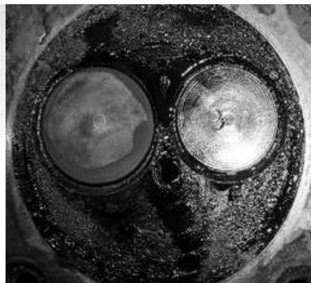
Fig. 3 Cylinderhead sedimentation after running with biofuels who are based on rape oil
