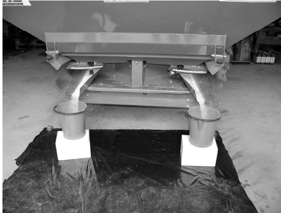
Figure 1 Measuring the mass flow rate in the laboratory
