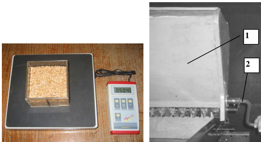
Fig. 7 The grain quantity and volume evaluation (left) . The calibration process (right) 1 – the grain thank; 2 – manual action of the distributor
