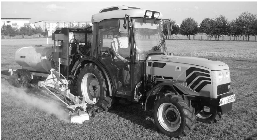
Figure 1 Hohenheim hot foam experimental machine mounted on a Deutz Agrocompact 75 during test application on lawn. Behind, the machine is linked with a 1000 litre water trailer.
