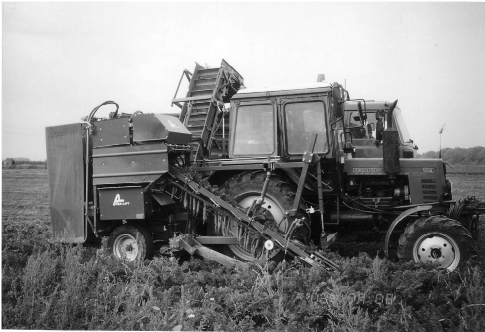
Picture 1 Root vegetable harvesting machine type ASA-LIFT-COMBI 1000
