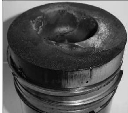
Fig. 5 Piston sedimentation after running with biofuels who are based on rape oil
