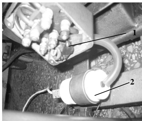
Fig. 5 The absorbed power transducer measured equipment: 1 – power convertor; 2 – transducer conection to the electric engine
