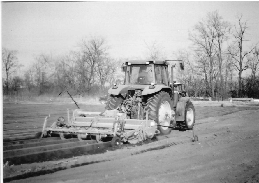
Picture 3 Ridge forming machine type RUMPSTAD FH4X75 RSF 2000
